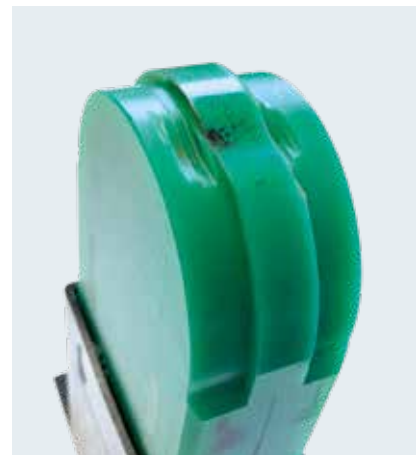
Possible wear patterns caused by overloading the Spann-Box®
